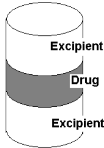
Figure 1: The prototype multi-layer compact, or tablet, considered here: a 3-layer version is shown. The tablet can be imagined as a typical cylindrical over-the-counter dosage form , e.g. an (unusual) aspirin tablet.
